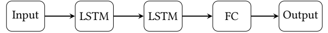
Figure 8: The architecture of the cascaded LSTM that used for single node data modeling.
